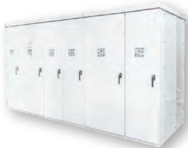
Pictured above: UL 891 / NEMA 3R, 480 / 800VAC, 6000A SWBD, single ended, with: cable input section, 5000A main, ACB feeder section, MCCB feeder section & SEL control section
