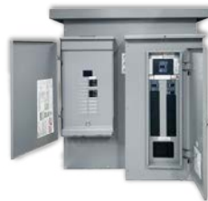
LV / 65kVA POWER CENTER, 600:480 3P & 600:120 1P DUAL SECONDARY
