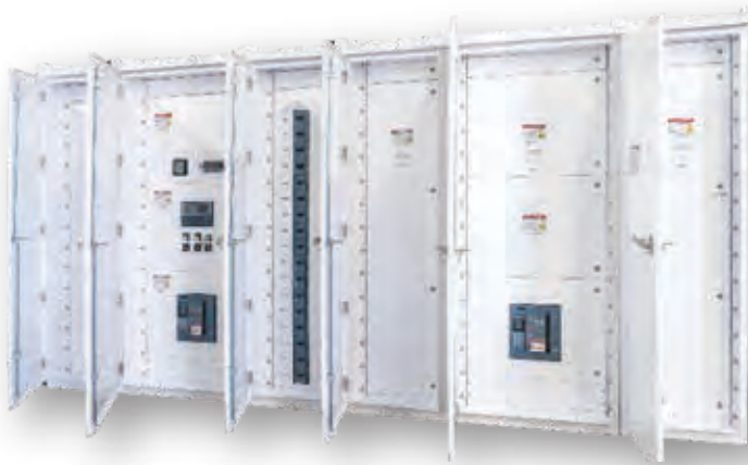
Pictured above: UL 891 / NEMA 3R, 480 / 800VAC, 6000A SWBD, double ended, with: cable input section, 5000A main, ACB feeder section, MCCB feeder, 2nd 5000A main, 2nd cable input section & SEL control section.
